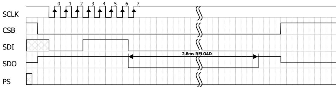
Figure 6: Reset command sequence SPI mode 3
