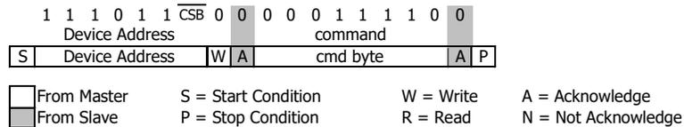
Figure 10: I<sup>2</sup>C Reset Command
