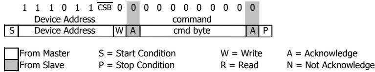
Figure 14: I<sup>2</sup>C ADC read sequence
