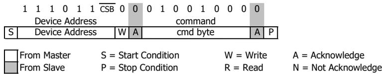
Figure 13: I<sup>2</sup>C Command to initiate a pressure conversion (OSR=4096, typ=D1)
