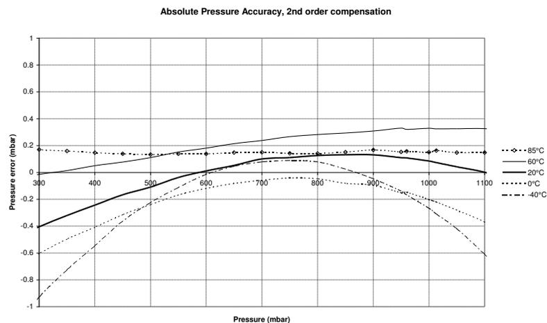
Pressure Error Accuracy vs temperature
